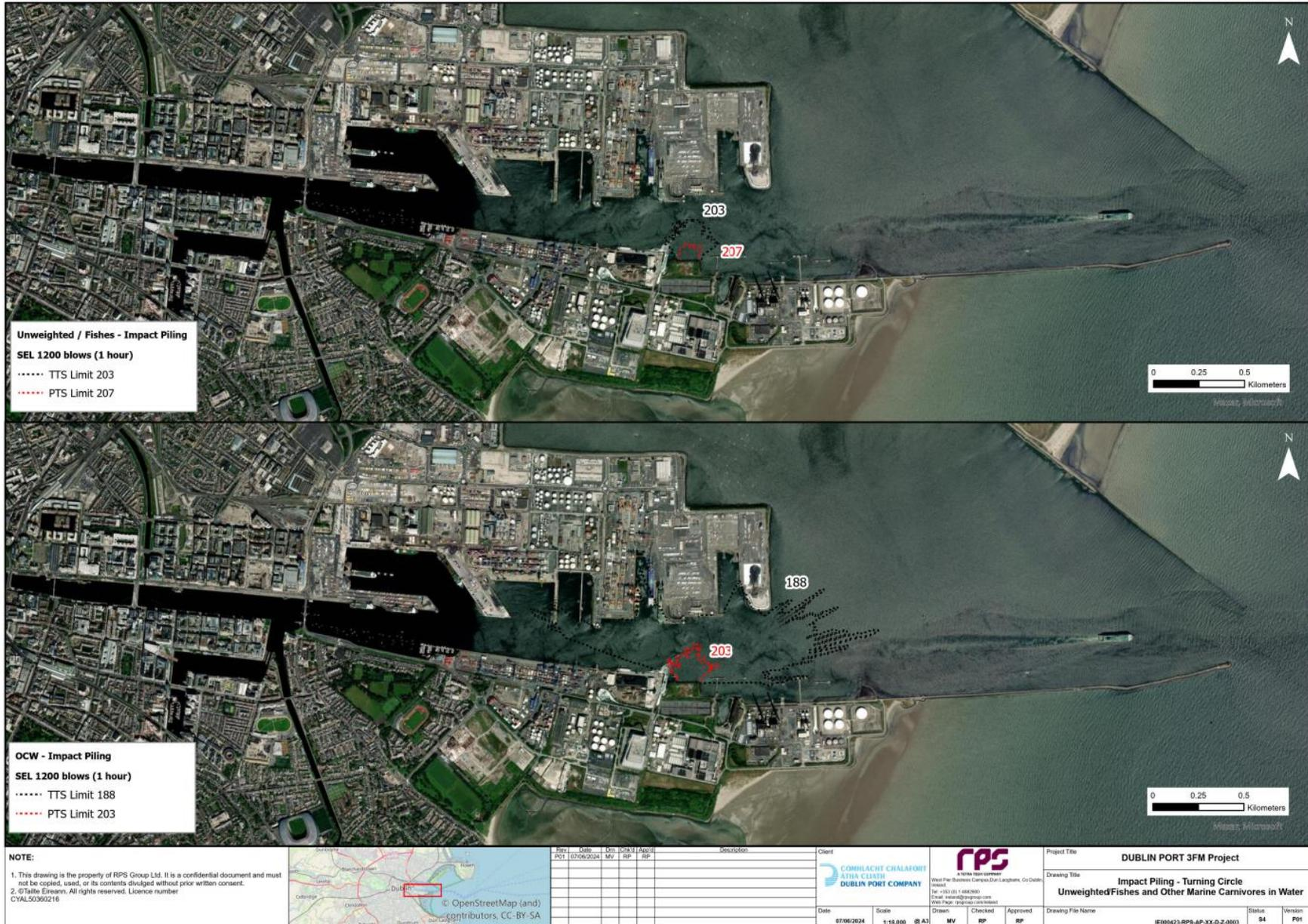
Figure 12.2.32. Impact piling, Turning circle, Fish (unweighted) and OCW hearing group.
