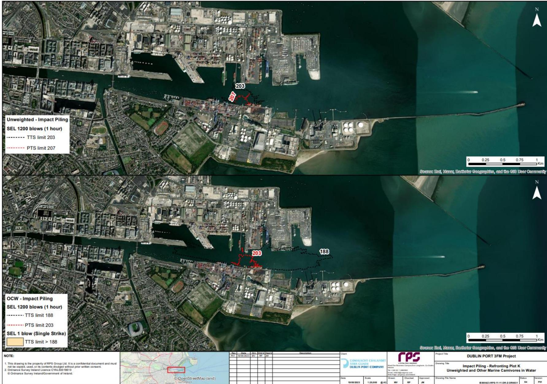
Figure 12.2.18. Impact piling, Area K, Fish (unweighted) and OCW hearing group.
