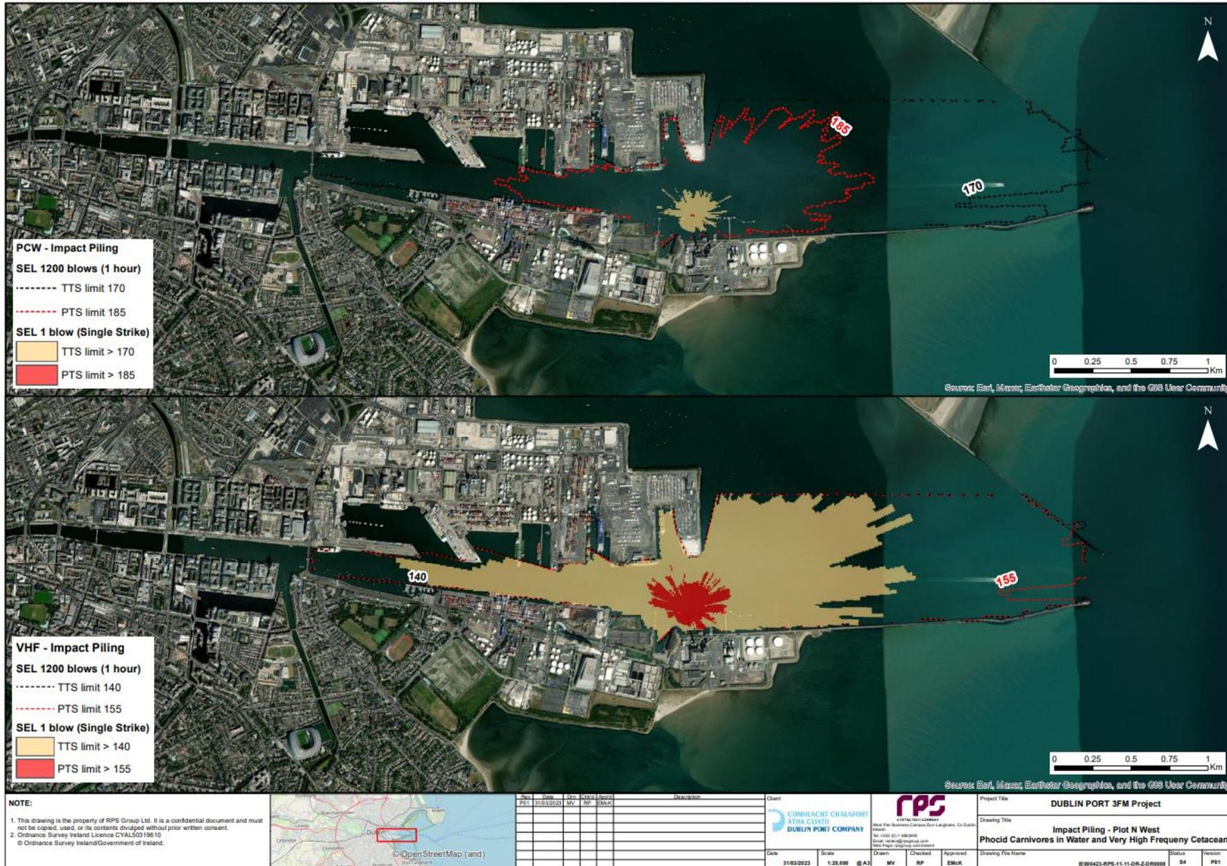
Figure 12.2.21. Impact piling, Area N west, Single piling rig, VHF and PCW hearing group.
