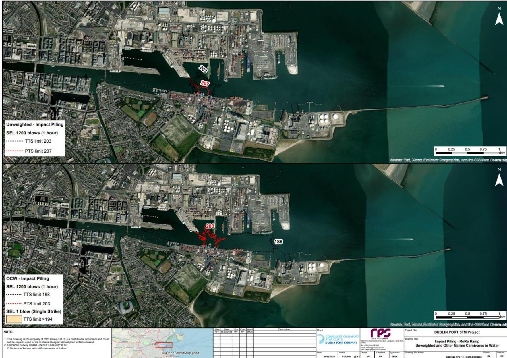
Figure 12.2.16. Impact piling, RO-RO ramp, Fish (unweighted) and OCW hearing group.
