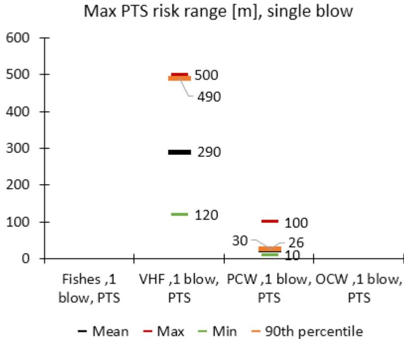
Figure 12.2.10. Overview of PTS risk ranges for a single blow for impact piling. Where no data is shown the range was under 5m.
