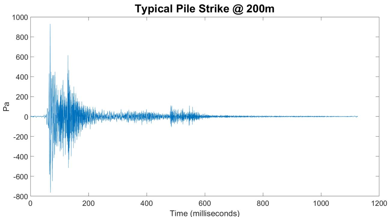
Figure 12.2.6 Typical piling strike measured at 200 metres from the source.
