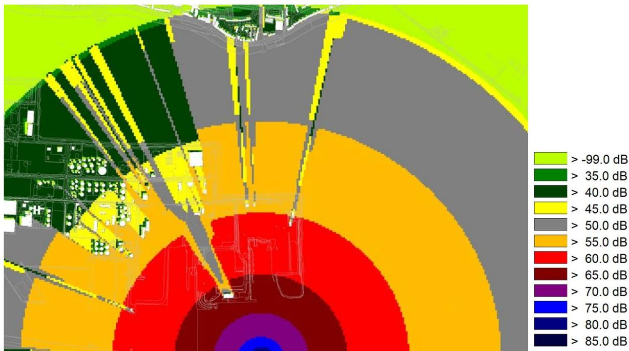
Figure 12.1.9 Noise Model of Construction Noise Levels at Clontarf
