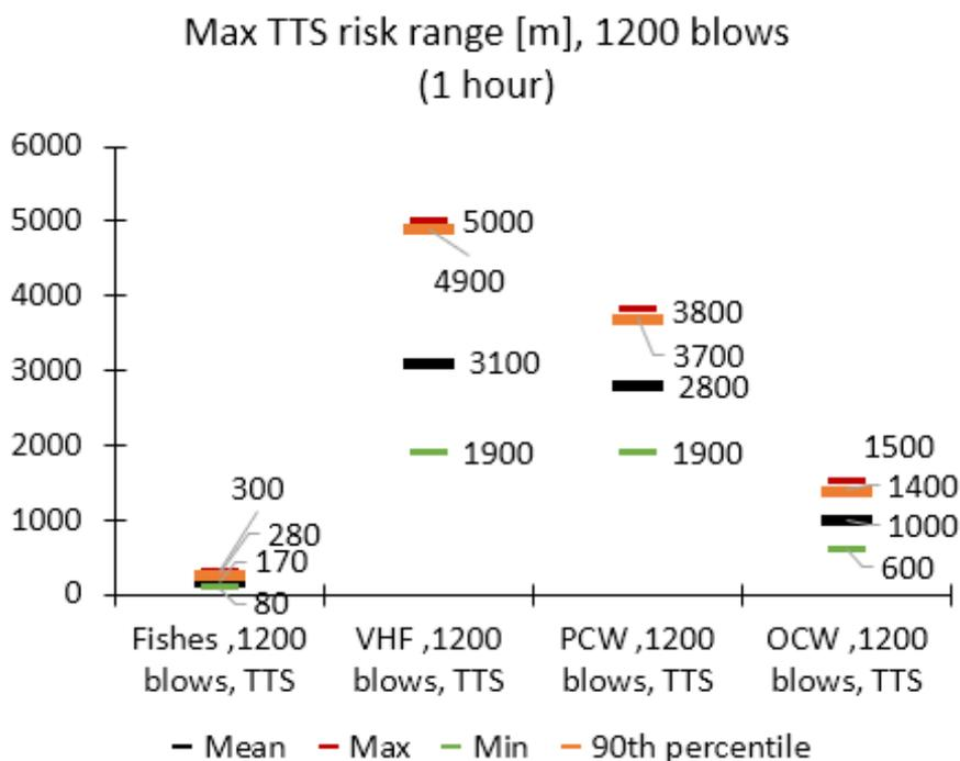
Figure 12.2.9 Overview of TTS risk ranges for 1200 blows for impact piling.
